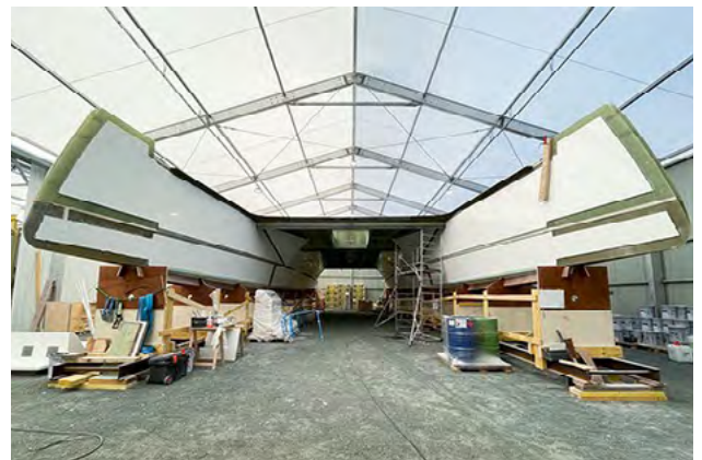
Figure 2 - Assembling Composite infused boat sides - Day One 75'
