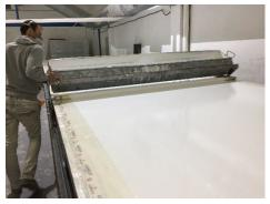
Figure 7: Pouring gel coat on the mold is still popular
