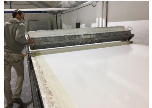
Figure 7: Pouring gel coat on the mold is still popular
